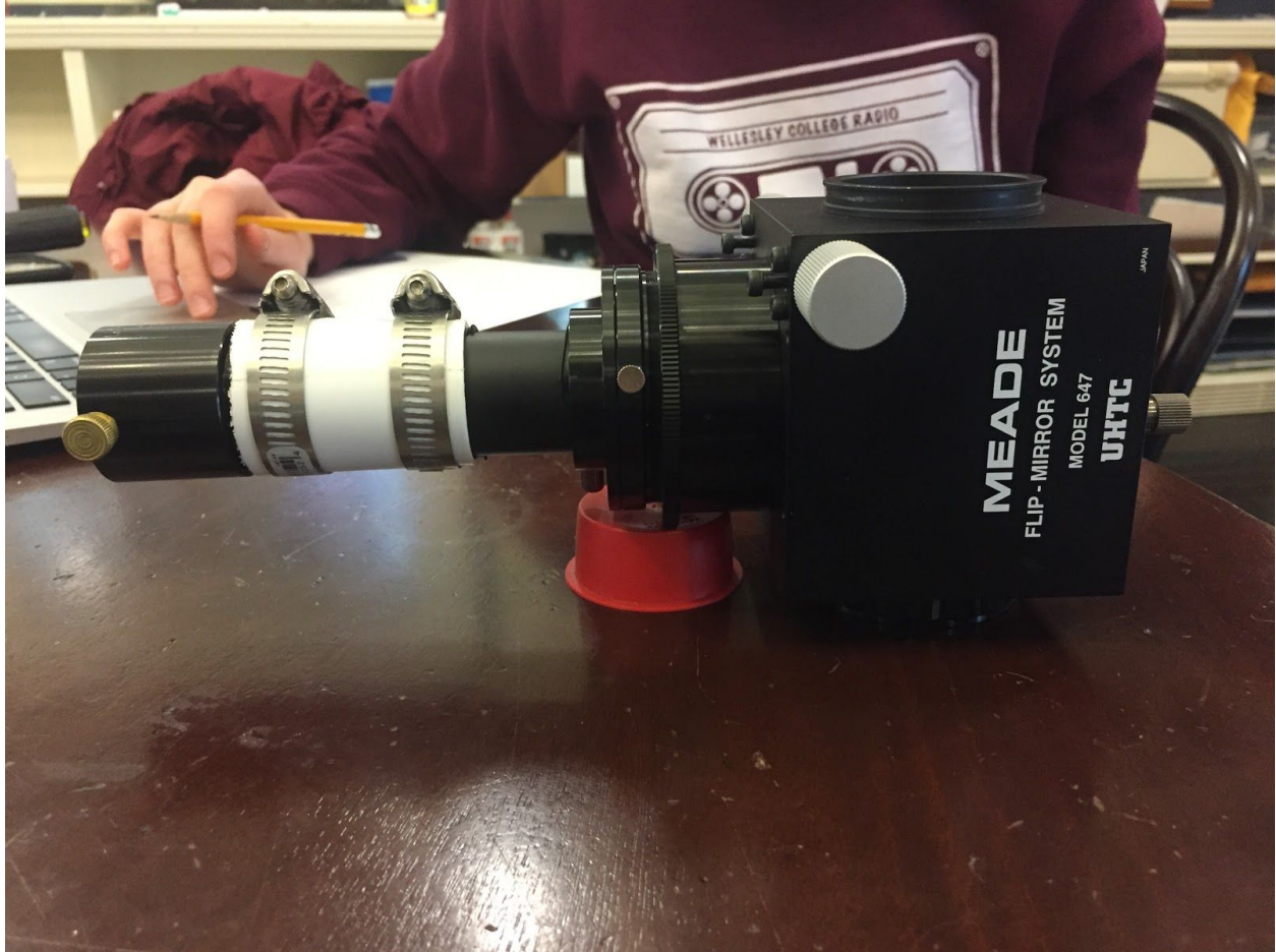
Figure 5: Guide camera system with Meade flip mirror system (side view). Guide camera not shown. Featuring Robin Siddall.
