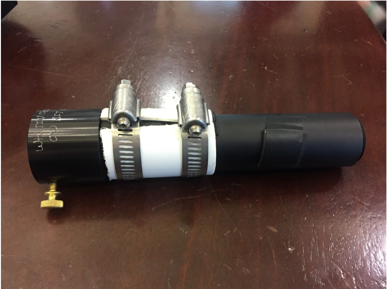
Figure 3: Guide assembly attachment with lens tube, 1" to 1.25" adapter, and PVC connection. Made flip mirror system and guide camera not shown.
