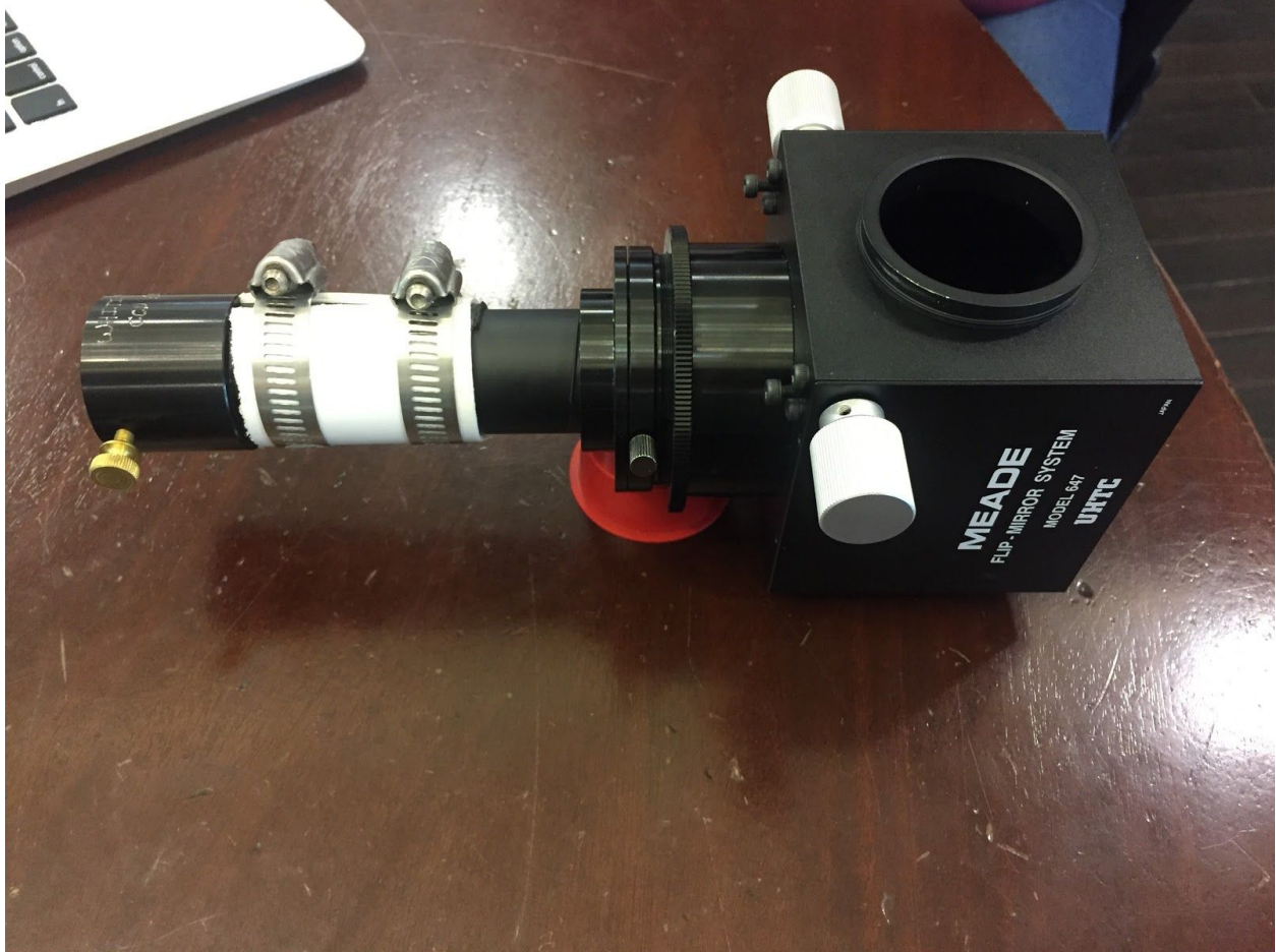
Figure 4: Guide camera assembly with Meade flip mirror system attached. Guide camera not shown.
